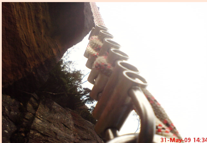
Descender with 1½ setup. The old rope was strategically placed in the ½ setup!
